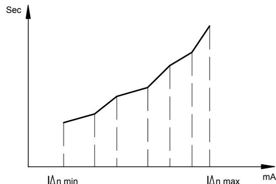
The test returns the residual current at which the circuit breaker trips.
